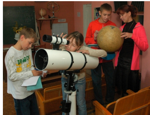
A Newtonian Telescope with a German equatorial mount.
